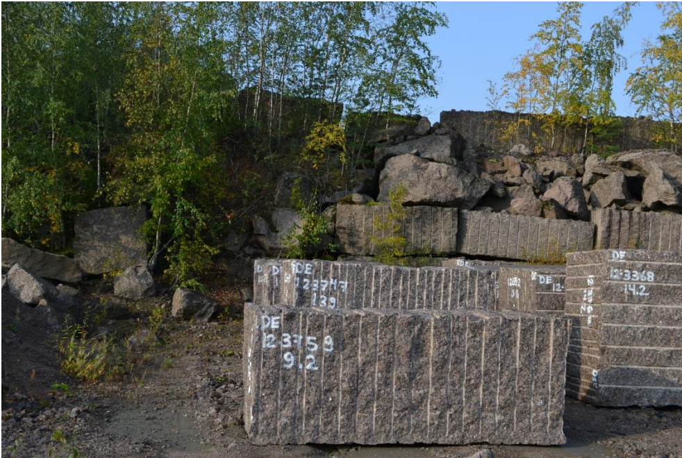
Figure 6. Granite block with special marks and personal ID number. This number carries information about the stone color and weight, among other things.
