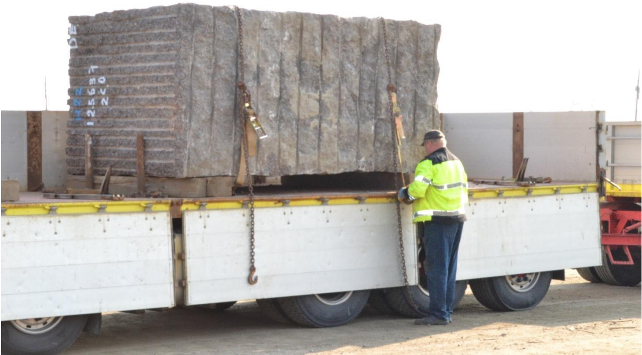
Figure 12 Fixing granite cargo to the truck. 2021
