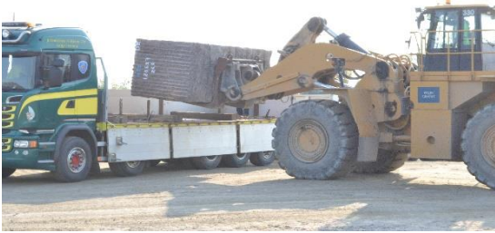
FIGURE 14. Loading of the block to a truck in the Palin granite quarry
