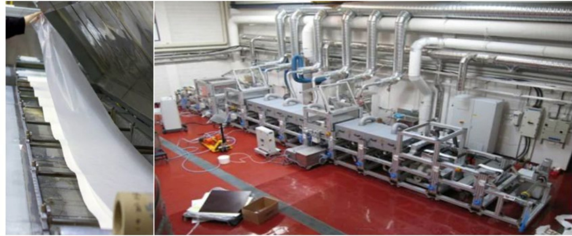
Surface Coating (SutCo) pilot line at VTT for preparing MFC films.
