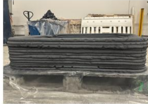
Layer geometry and buildability check
